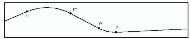
Figure 10 - Sample Polyline Feature with two Curves
