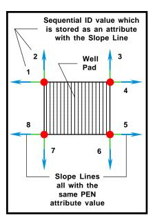
Figure 4 Well Pad Layout and associated Slope Lines
