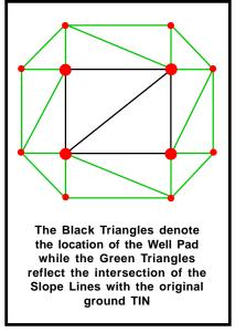
Figure 5 Polygons created using Polygons from Slope Lines
