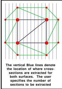
Figure 6 Extraction of Cross-Sections for determining Cut/Fill Volumes
