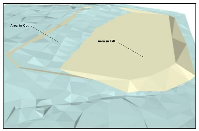
Figure 16 ArcScene Display of the Original Ground and Well Pad Polygons
