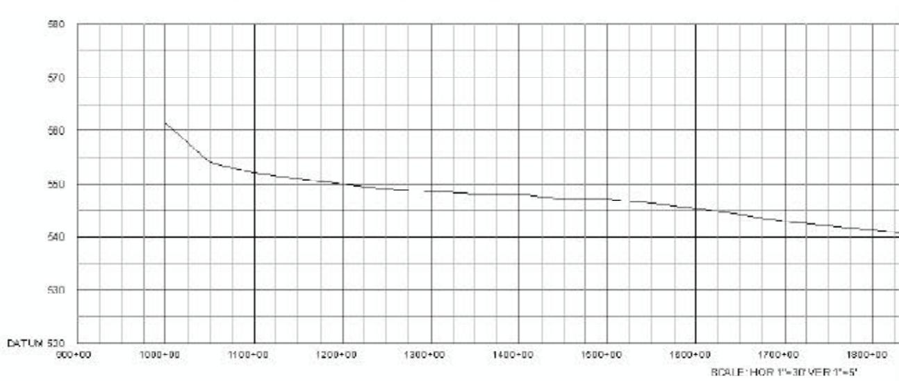
Figure 10 - Profile with the parameter Type of Grid set to Full Grid w/ Full Stations
