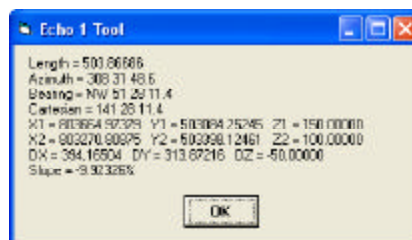
Figure 5 Echo Information Between Two Points
